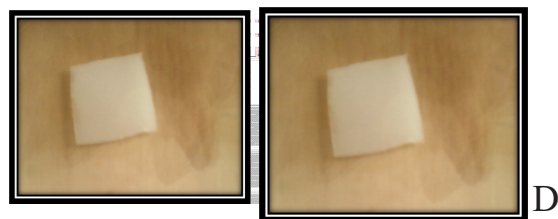
Figure 3: Degradation of films (before & after) by fungus A. niger
