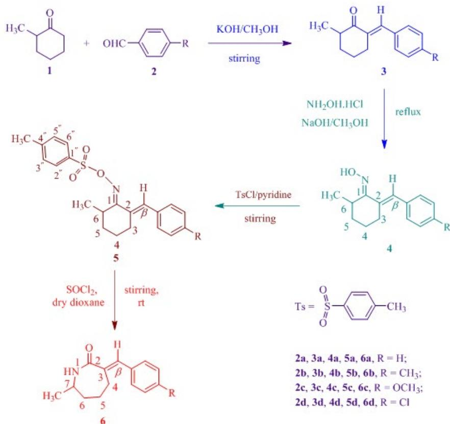
**Scheme 1:** Synthetic route for the preparation of *(E)*-3-arylidene-7-methylazepan-2-ones (**6**)
